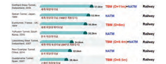
[그림 8] 7 Longest Tunnels in the World (NATM and TBM)
